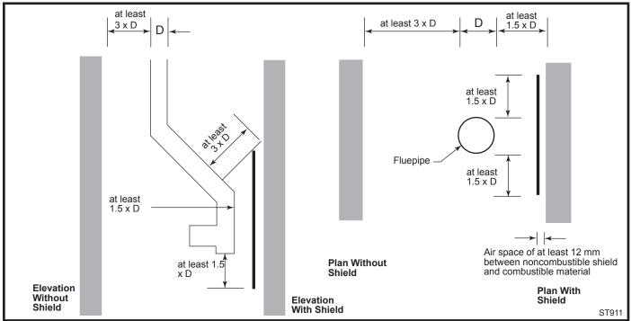
Fig. 13 Connecting fluepipe clearances.
